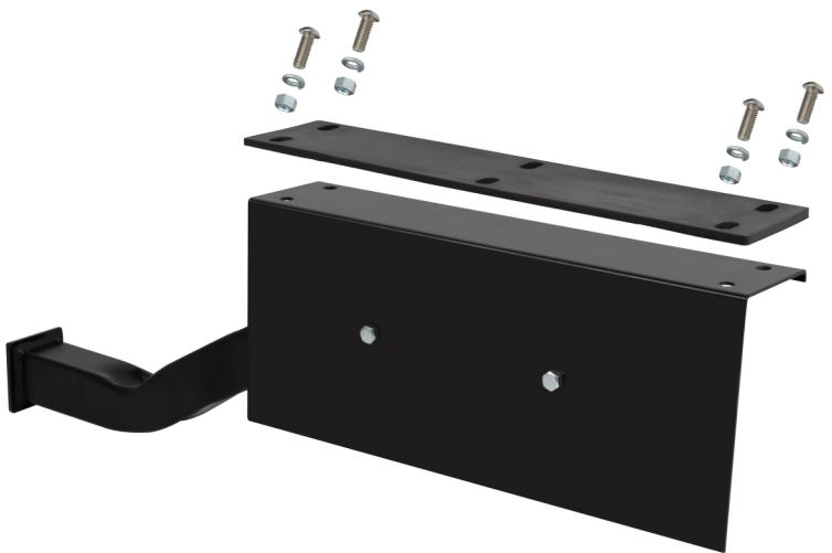
**Installation Notes:** Before installing this rear bracket, front bracket must be secure and in place. The fender must also be level with truck frame. Align rubber stripping on top of bracket plate. Place rear bracket under rear portion of half tandem fender or center of full tandem fender, install and bolt to frame. Some drilling may be necessary to maintain the level position of the fender. Failure to use the included rubber stripping voids all warranties. **DO NOT USE GRADE 8 BOLTS.**
